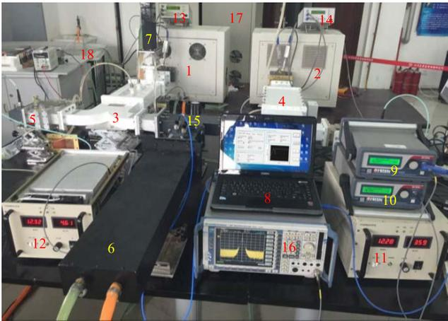
Fig. 9. Power combining system (1 and 2: the magnetrons with electromagnets, 3–5: circulators, 6 and 7: water loads, 8: laptop, 9 and 10: microwave solid-state sources, 11 and 12: microwave power amplifiers, 13 and 14: microwave power meters, 15: waveguide tee combiner, 16: spectrum analyzer, 17: magnetron dc power supply, and 18: water tank).
