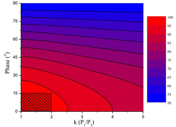
Fig. 6. Power combining efficiency with respect to input power ratio and phase difference.
