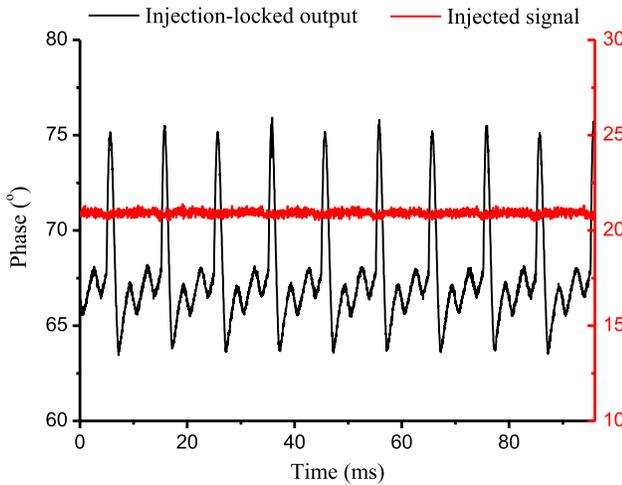
Fig. 4. Phase jitters of the injection-locked magnetron microwave output and the injected signal.
