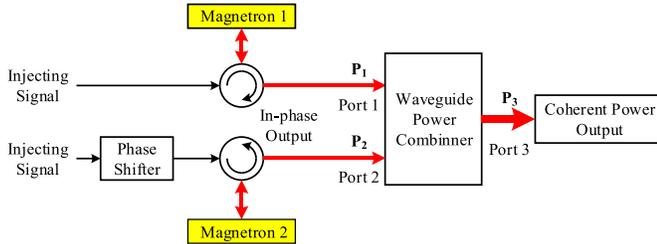
Fig. 5. Principle diagram of dual injection-locked magnetrons applied to microwave power combining.
