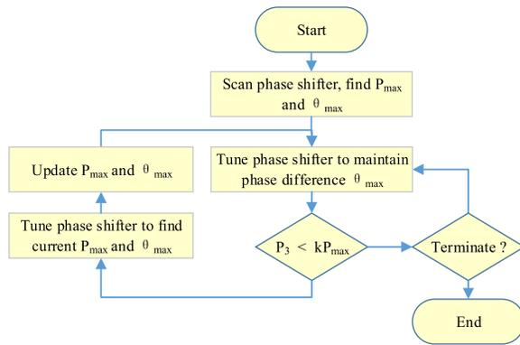
Fig. 8. Program flowchart of phase controlling.
