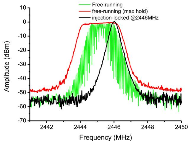
Fig. 2. Spectrum of the magnetron microwave output at various states.
