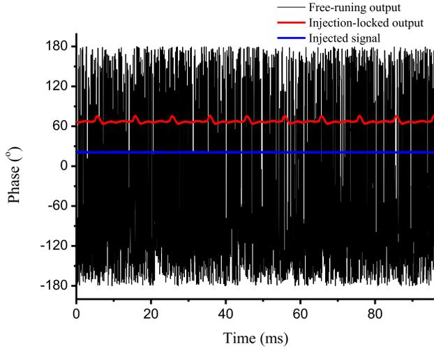
Fig. 3. Output microwave phase jitters of free-running and injection-locked magnetrons.
