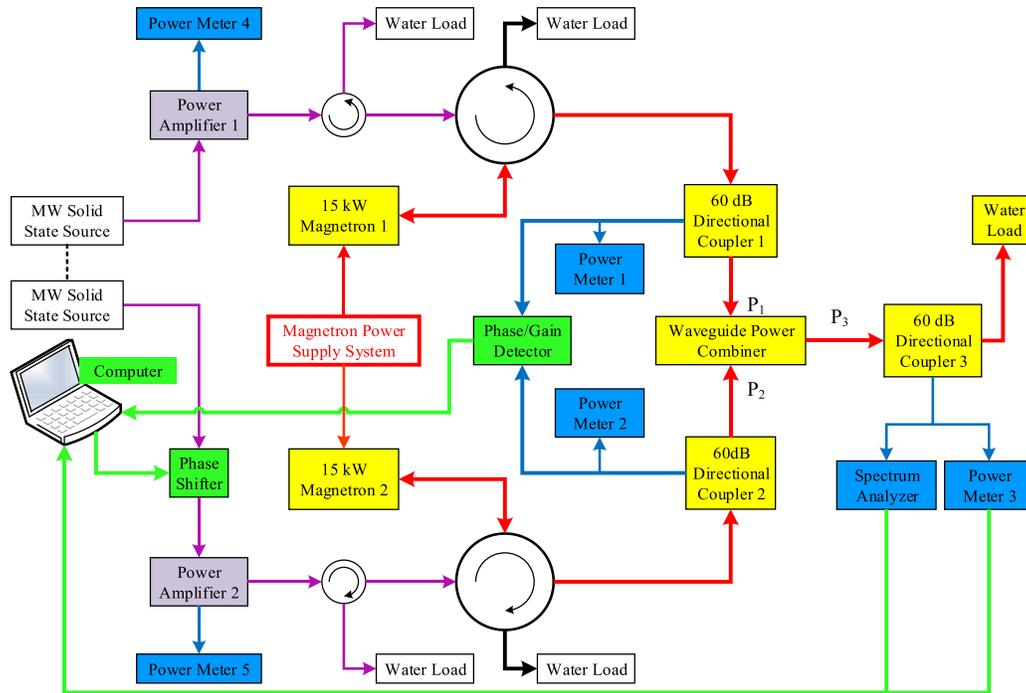
Fig. 7. Schematic of the microwave power combining system based on two-way injection-locked 15-kW CW magnetrons.
